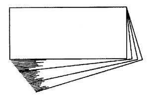
Without removing paste, bills pick failure will occur.
